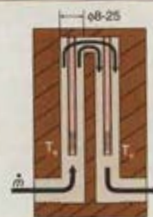
FIGURE 3. Typical sensor configurations of industrial thermal mass flowmeters. All dimensions are in millimeters. T_v indicates the heated velocity sensor. T_s indicates the temperature sensor. \dot{m} is the total mass flow rate.
